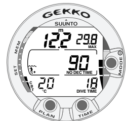
Fig. 3.10. Ascent Rate Indicator. Three segments.
