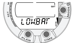
Fig. 3.2. Startup II. Battery power indicator.
