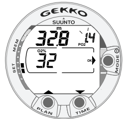
Fig. 4.17. Setting Nitrox parameters. Oxygen percentage is 32%, oxygen partial pressure limit is 1.4 bar. The equivalent maximum depth is displayed as 32.8 m [107 ft]. Press scroll buttons to change oxygen percentage and to set oxygen partial setting value. Accept settings by pressing MODE (OK).
