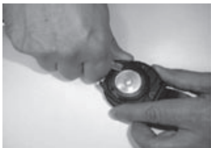
Fig. 5.2 Opening of the securing ring.
