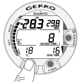
Fig. 3.8. Bookmark activation. An annotation, Bookmark, is placed in the profile memory during a dive by pressing PLAN button. Note Logbook symbol.
