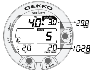
Fig. 3.13. A Mandatory Safety Stop. You are advised to make a Mandatory Safety Stop in the depth zone between 6 m and 3 m [20 ft and 10 ft]. Pressing TIME button shows alternative display.
