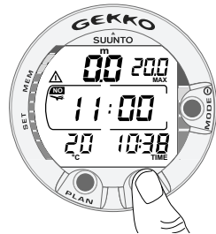
Fig. 3.28. Surface interval, no-flying time. Pressing TIME button twice will show no-flying time, indicated by an airplane icon.
