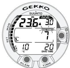
Fig. 3.15. Decompression dive, below floor. Upward pointing arrow, blinking ASC TIME label and an audible alarm tell you to ascend. Minimum total ascent time including safety stop is 7 minutes. Ceiling is at 3 m [10 ft].
