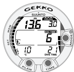
Fig. 3.16. Decompression dive, above floor. Upward pointing arrow has disappeared and ASC TIME label has stopped blinking, which means that you are in the decompression range.
