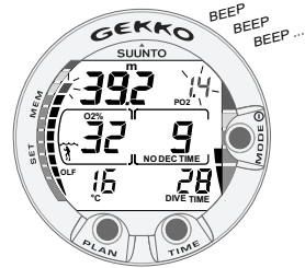
Fig. 3.23. Oxygen partial pressure and OLF displays. There is an audible alarm as oxygen partial pressure is greater than 1.4 bar or set value, and/or the OLF has reached 80% limit.
