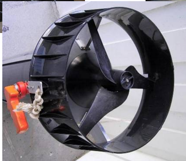
Propeller-Schutz montiert (shroud, duct)
